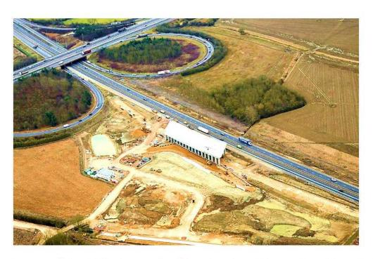
The carriageway of the A428 close to the Girton junction will be realigned in early May. Moving traffic at this location allows us to complete work on the final alignment of the eastbound carriageway, which will eventually pass through the span of the new bridge being built at the side of the A428 (pictured above). We expect traffic to be using this new route at the end of July.
